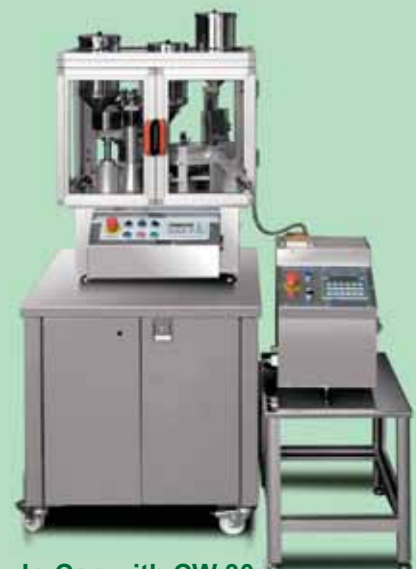
In-Cap with CW 30 check weigher in line
